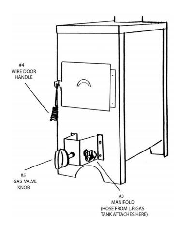
(7) LIGHTING INSTRUCTIONS: To light stove, turn on gas supply at tank. To open stove valve, DEPRESS KNOB (Part #5), turn 1/8 turn to the left, and IMMEDIATELY place a lighted match near the top of the burner. If flame goes out, turn off stove valve immediately and repeat instructions.
