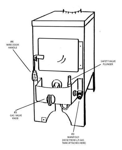
(7) LIGHTING INSTRUCTIONS: To light stove, turn on gas supply at tank. To open stove valve, DEPRESS KNOB (Part #5) and turn 1/8 turn to the left. Place a lighted match near the top of the burner and DEPRESS PLUNGER for approximately one minute, or until stove stays on after plunger is released. If flame goes out, turn off stove valve immediately and repeat instructions.
